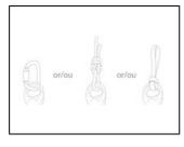
Swivel and auxiliary attachment point allow the use of carabiners, ropes, or slings for easier rigging.
